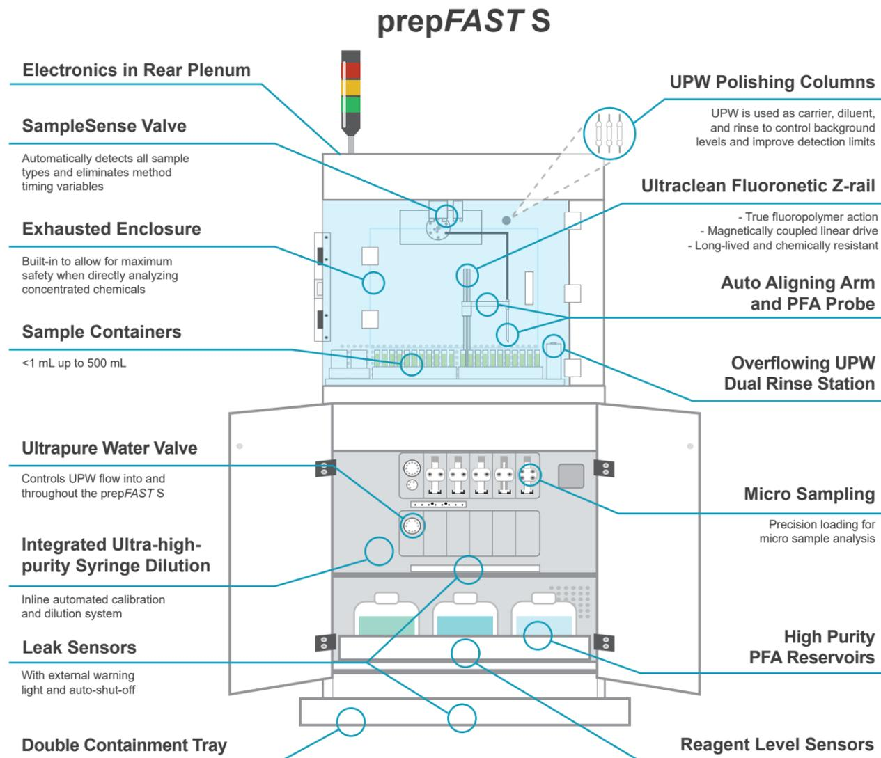
Figure 2. prepFAST S features diagram.
